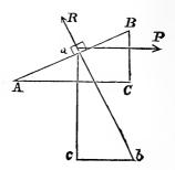
The body is kept at rest by three forces, P acting parallel to the base of the plane, W acting vertically downwards, and R the reaction of the plane.
